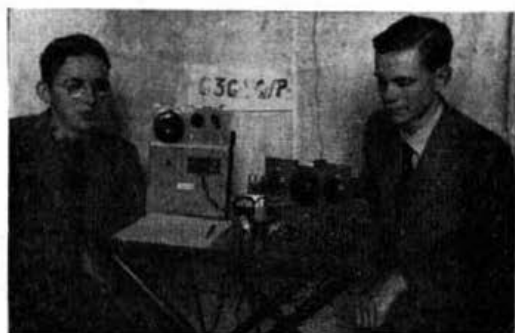
The rig at G3GYQ/P, showing (left to right) transmitter on top of power supply box meter, 100 kc/s. standard and receiver, G3GYQ and G3EIX are at left and right respectively.
